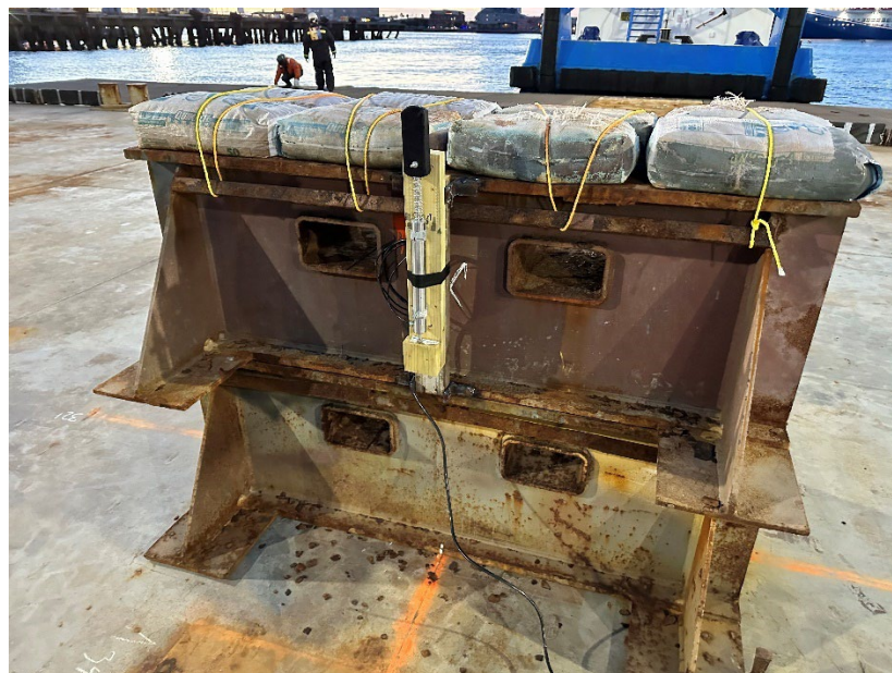
Figure 17: Keel Block Indicator Installed
