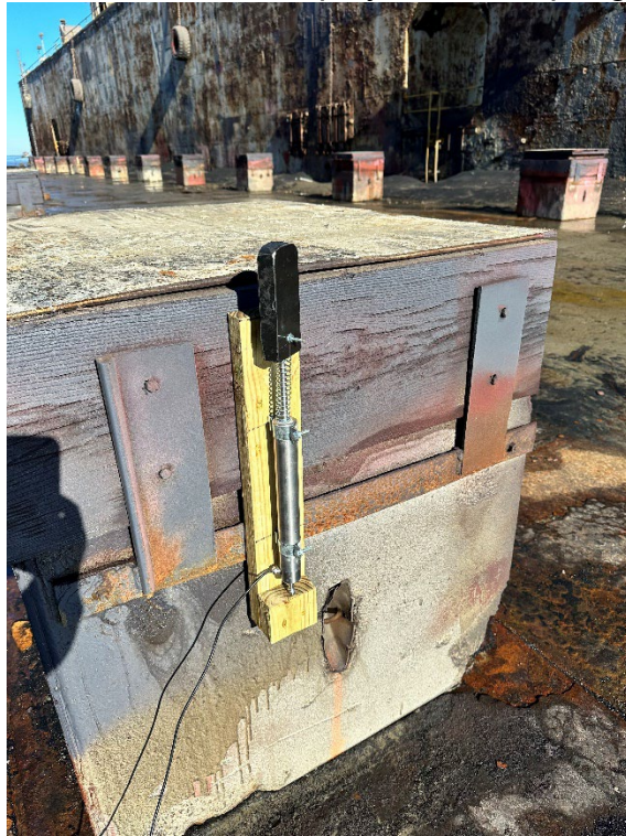
Figure 14: Sensor mounted on the block, showing mechanical extension after undocking.
