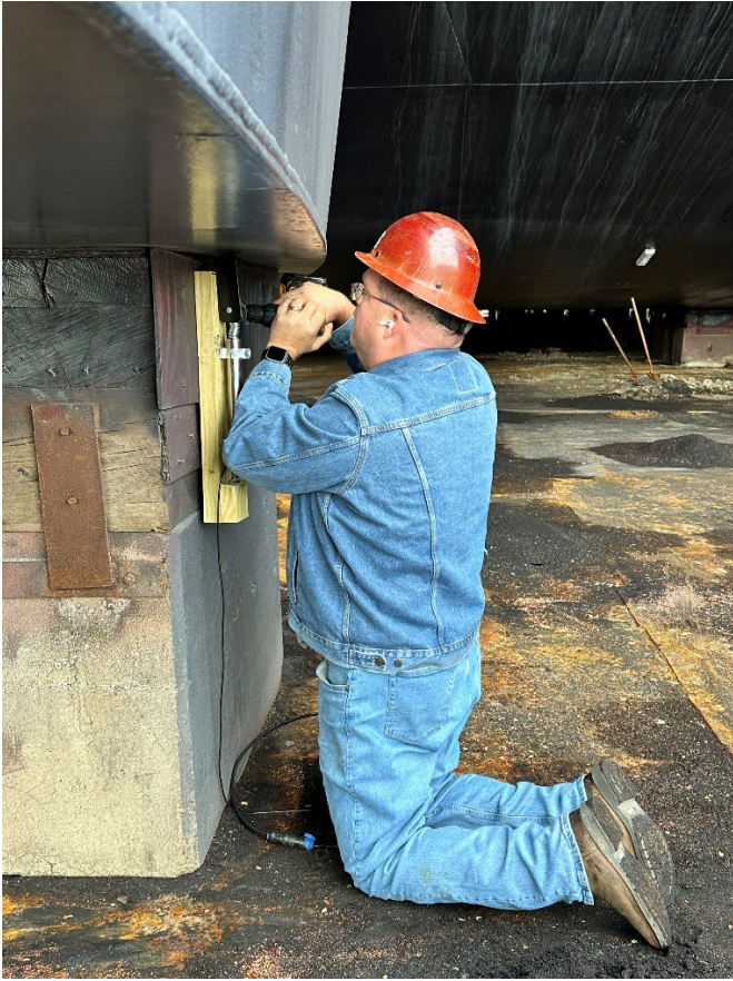
Figure 8: DMC attaching the sensor to a block.
