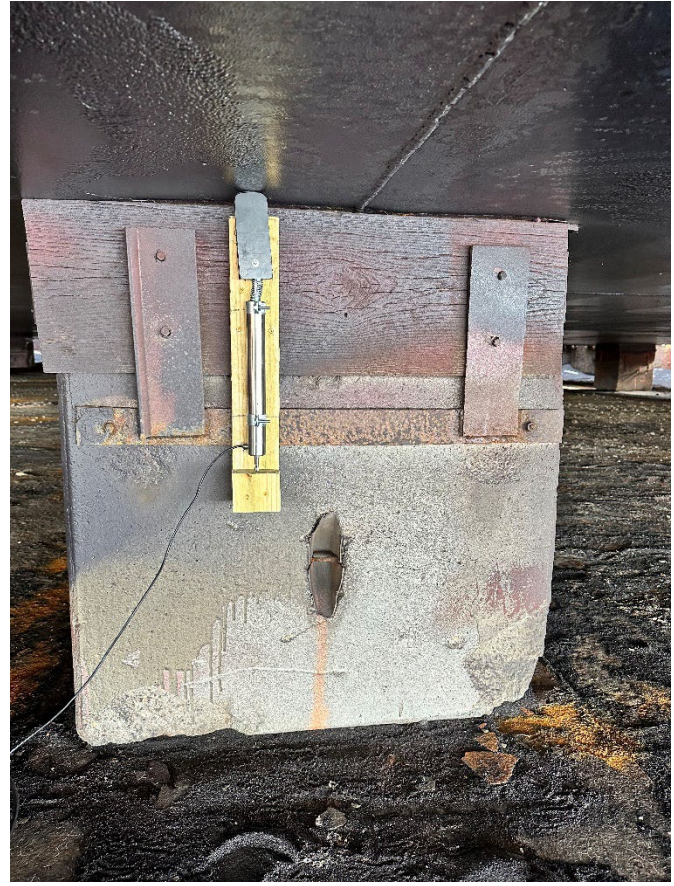
Figure 9: Sensor installed on a block.
