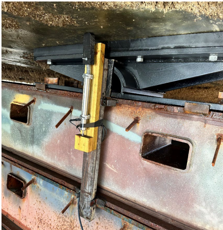
Figure 2: Linear Position Sensor Against Ship Hull
