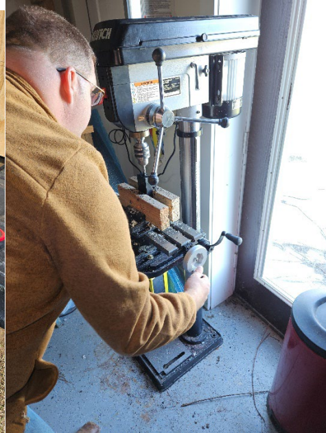
Figure 5: DMC machining HDPE probe
