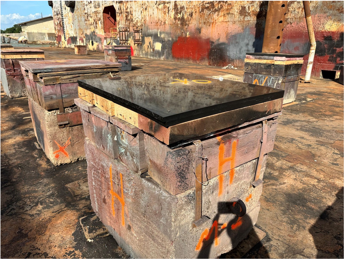
Figure 4: Docking 2 HDPE Keel Block 1
