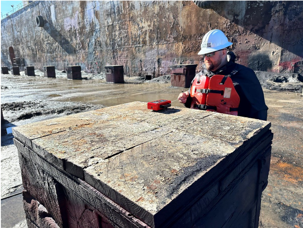
Figure 22: Alex Stiglich, DMC performing a friction test on a wooden cap.
