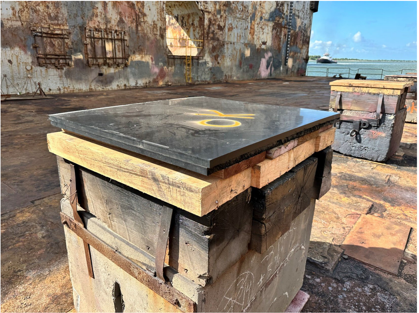
Figure 5: Docking 2 HDPE Keel Block 2
