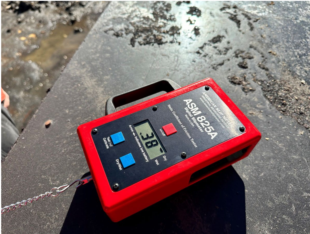
Figure 23: Slip meter utilized for friction testing, reading a coefficient of 0.38
