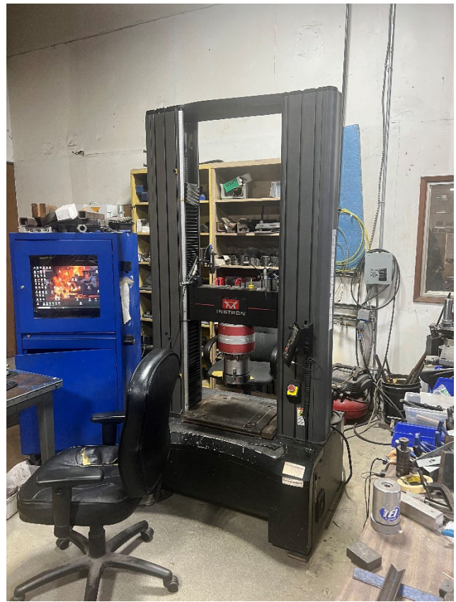
Figure 21: Equipment Used for Splitting Tensile Tests
