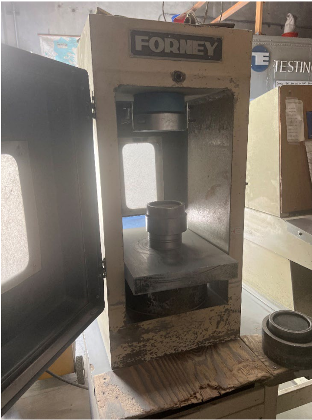
Figure 20: Equipment Used for Compression Tests
