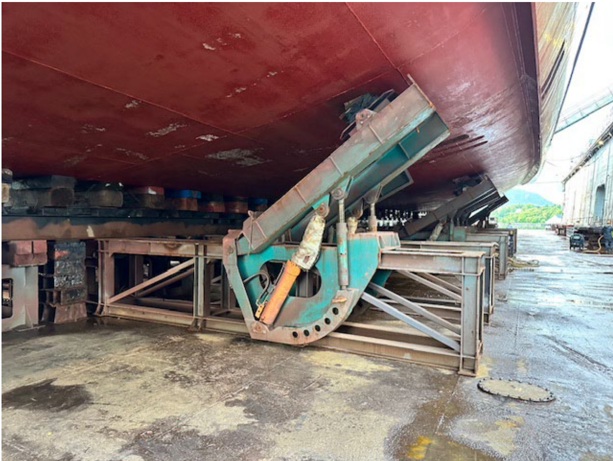
Figure 3: Photo of Bilge Support Arms
