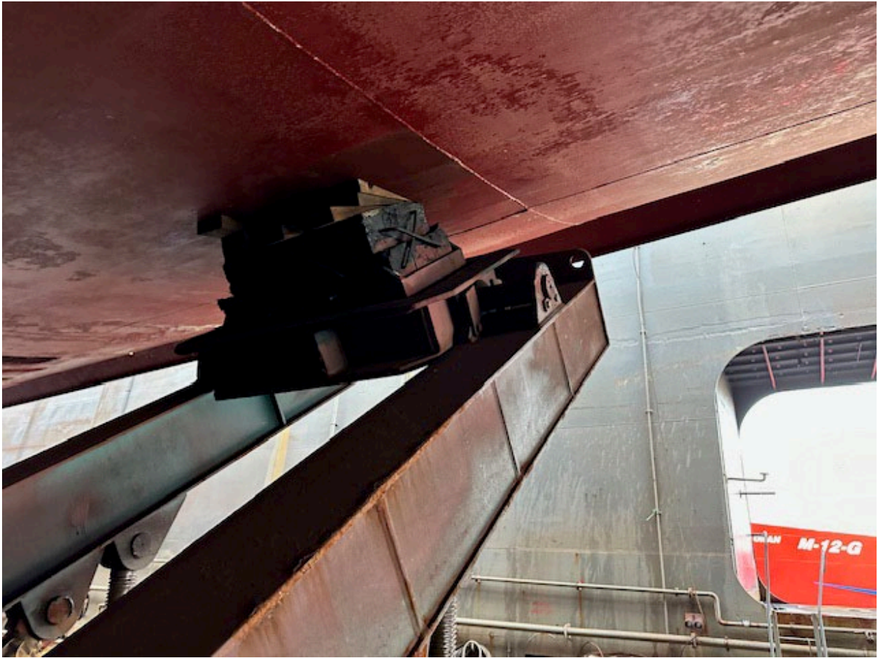
Figure 4: Photo of Bilge Support Arms Upper Rotating Face
