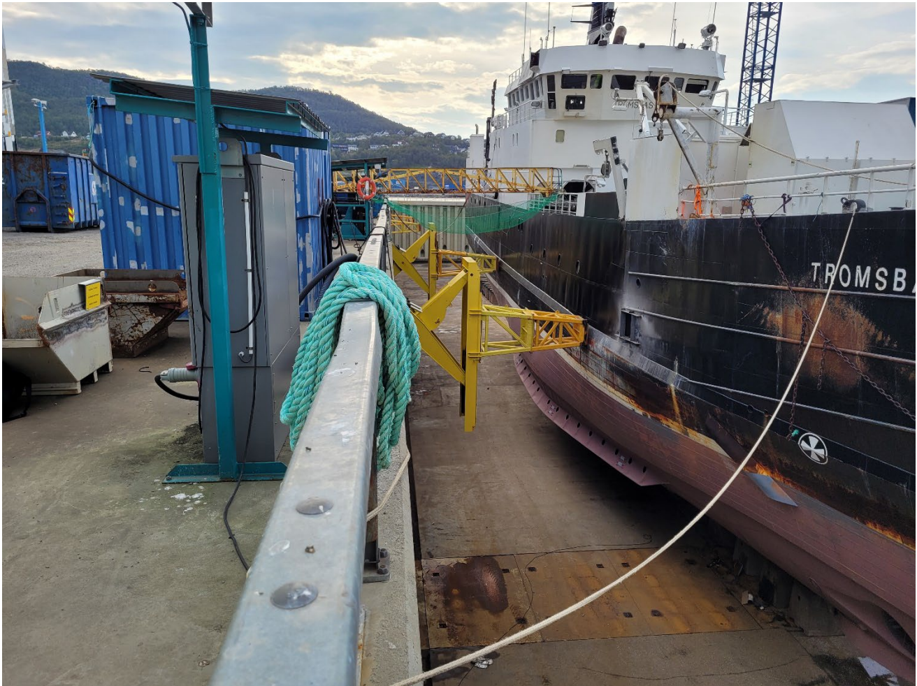
Figure 14: Photo of Sidewall Support Arm Showing Typical Vessel Support
