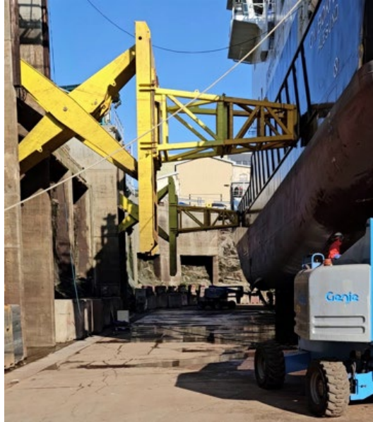
Figure 2: Photo of Side Support Arms
